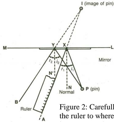
Figure 2: Carefully sight along the ruler to where the pin's image meets the paper.
